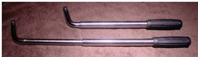
Emergency Breaker Bar in normal and extended positions
